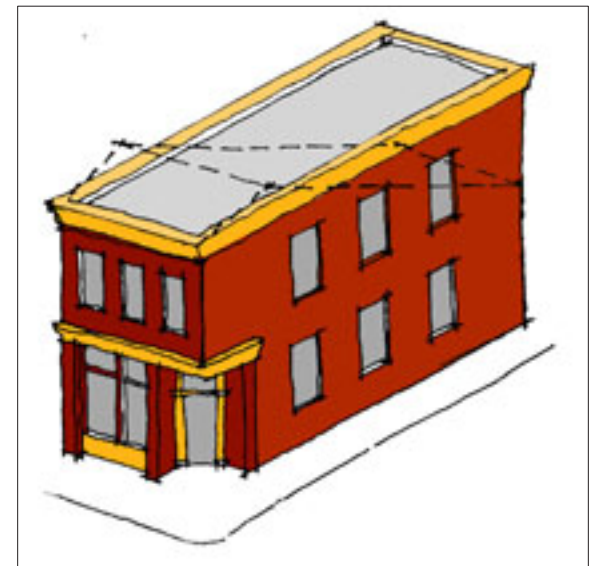
Inappropriate alteration: Changing the primary roof form to allow for additional headroom on the second floor.
