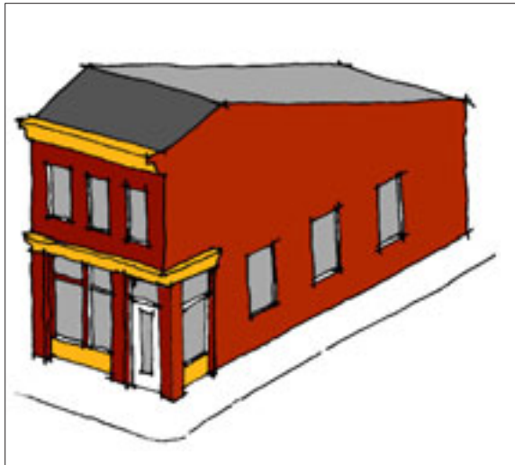
Inappropriate alteration: Changing corner entrance configuration.
