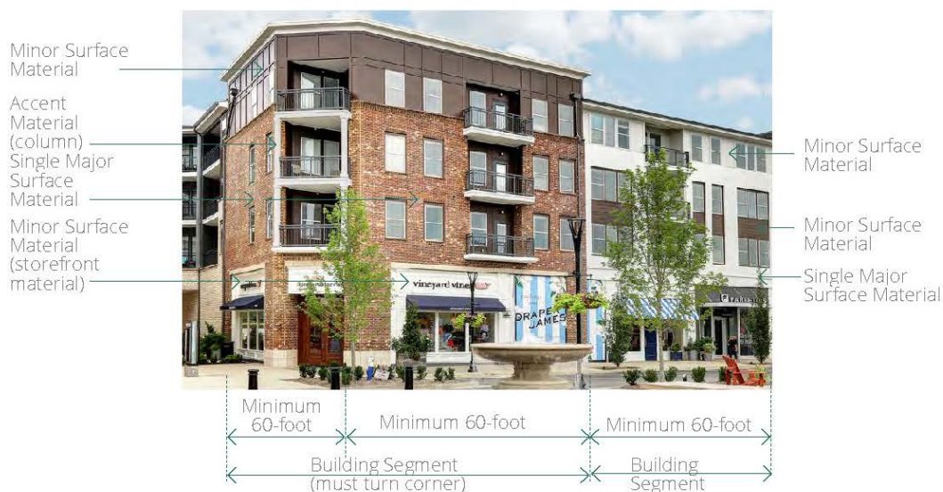
Figure 10.16.4-33 Major and Minor Materials on a Facade
