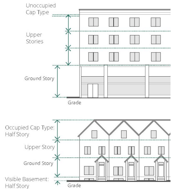
Figure 10.16.6-66 Measuring Stories with Floor-to-Floor Height
