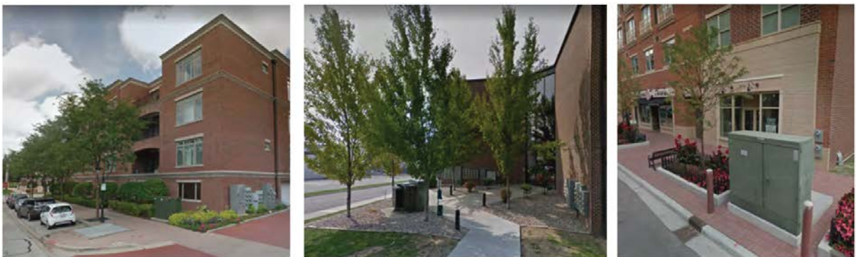
Figure 10.16.4-46 Examples of Poorly Located Utility Appurtenances without Screening on Primary Streets: NOT PERMITTED
