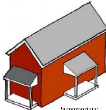
Inappropriate: New side porch is too large.
