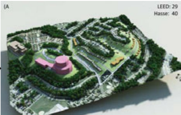
Figure 5.9 (left) Enlargement from worksheet of 3-D design concept (concept A, site 2) with evaluation scores and land use color coded to present a more realistic development model. A larger version of the worksheet can be found in Appendix 10.3.
