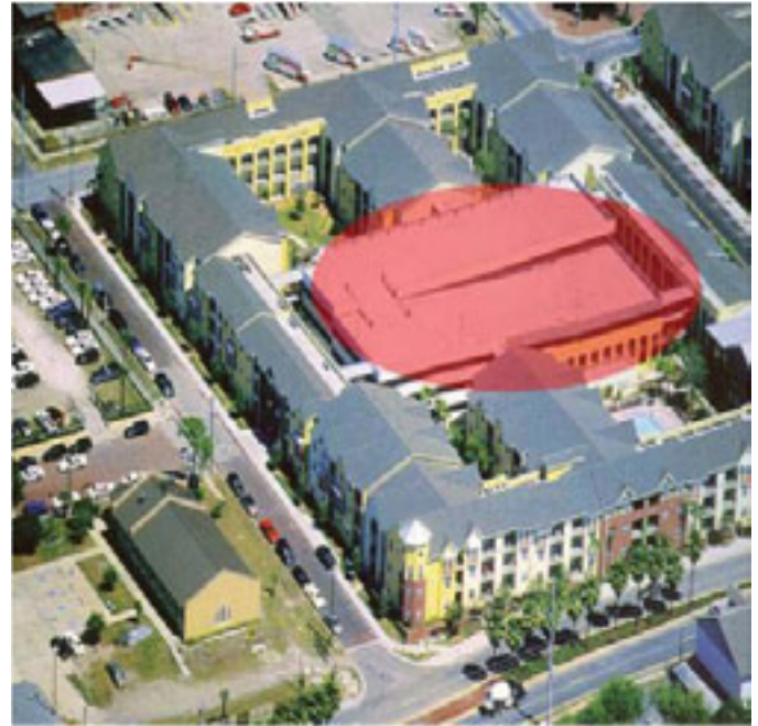
Figure 6.8 An example of an internal parking structure (highlighted in red) where parking is placed to the interior of a development block.
