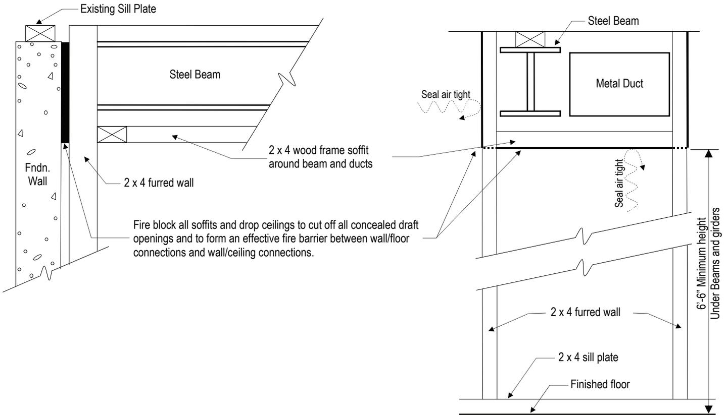
**SOFFIT FIRESTOPPING DETAIL**
