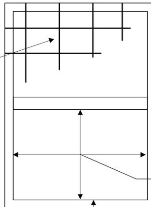
The emergency escape window must have a minimum opening of 5 square feet. The opening must be at least 20" wide and the height of the opening must be at least 24".
